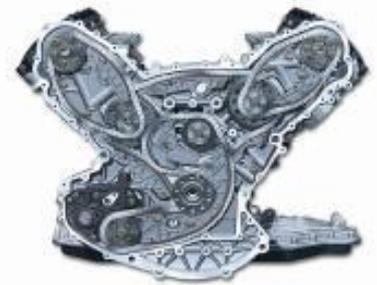
*Complex timing and oil-pump drive chains*
